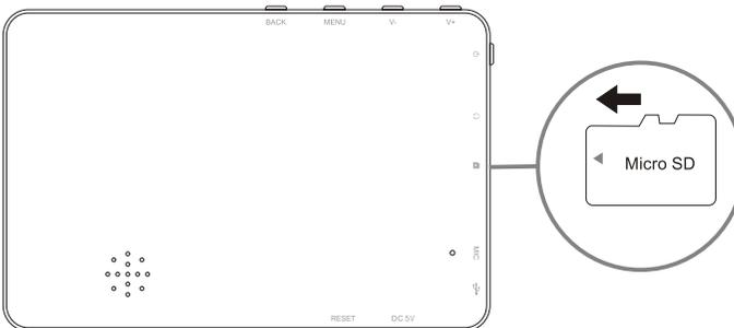
When you want to remove the Micro SD card, touch the SD Card icon in the Notification bar, and select and touch “sdcard is mounted”, then press the card in the slot and it will pop up, take it out gently.
